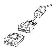
4. Tighten the screws on all the connectors.
