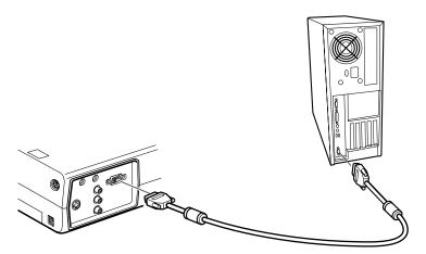
Tighten the screws on all connectors.
