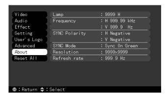
When the image source is a computer, the About menu displays information about the projector's horizontal and vertical frequency, lamp hours, and computer connection.
