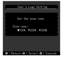
7. Use the Enter button on the remote control to select a zoom rate (display size), and then press Enter.
