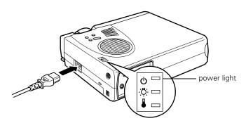
2. Plug the other end of the cable into a grounded electrical outlet.
