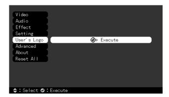
The User's Logo feature allows you to transfer any image on your computer to the projector, and then use it as the screen displayed when the projector is not receiving a signal. You can also set it as a startup screen or to be displayed when you press the A/V Mute button on the remote. The image can be a company logo, slogan, photograph, or another other image you want to use.
